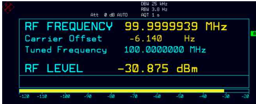
Fig. 11 RF Level measurement display
